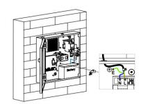
Place the battery as shown in the figure, and use the fixing plate and M3X5 crohsshead screw to fix it.
