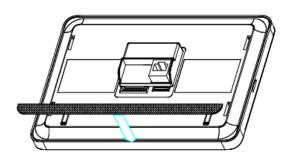
Align the edge of the silicone non-slip mat to the back of Indoor Monitor.
