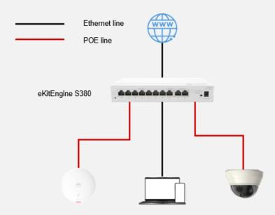
Huawei eKitEngine S380 series Multi-Service Gateway include various models, such as those with 4 downlink GE electrical ports, 8 downlink GE electrical ports (PoE/non-PoE ports), or GE uplink ports. With features like easy installation and deployment, as well as flexible Ethernet networking, the products can be widely used for indoor coverage in SME markets such as SOHO enterprise office, economic hotels, factories, primary and secondary education, and building security.
