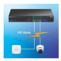
**PoE Power** This managed PoE++ switch comes with eight PoE++ ports that can supply up to 180W of PoE power.
